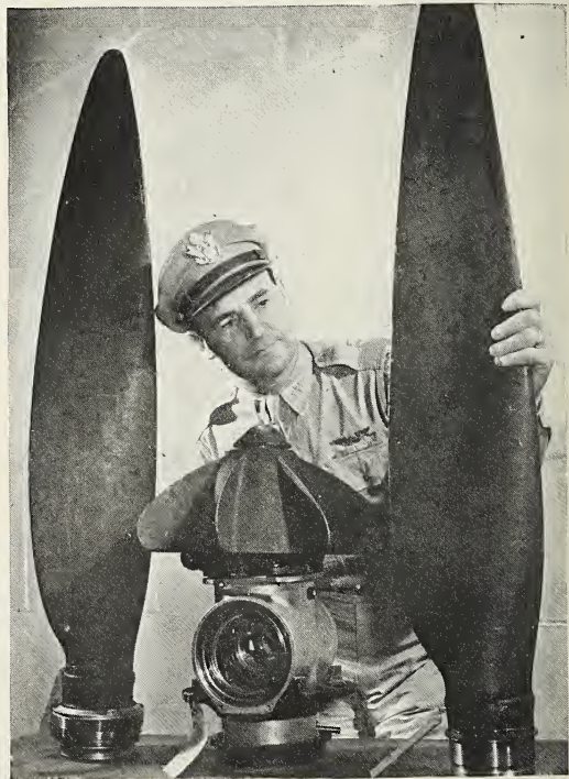
The pitch of these German Argus prop blades is controlled automatically by the ribbed rotatable spinner which reacts with changes in air speed. Wooden-bladed, the prop is used on low-power engines.
